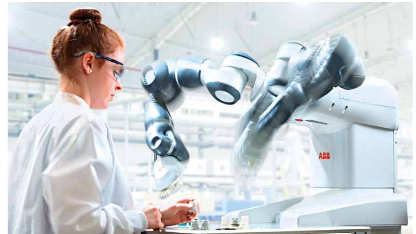
YuMi can take on assembly tasks with two hands. It can both touch and see. The robot has special flexible hands and an innovative sense of touch that make it a safe colleague for humans.
