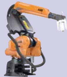
Paint robot: IRB 5400-22
