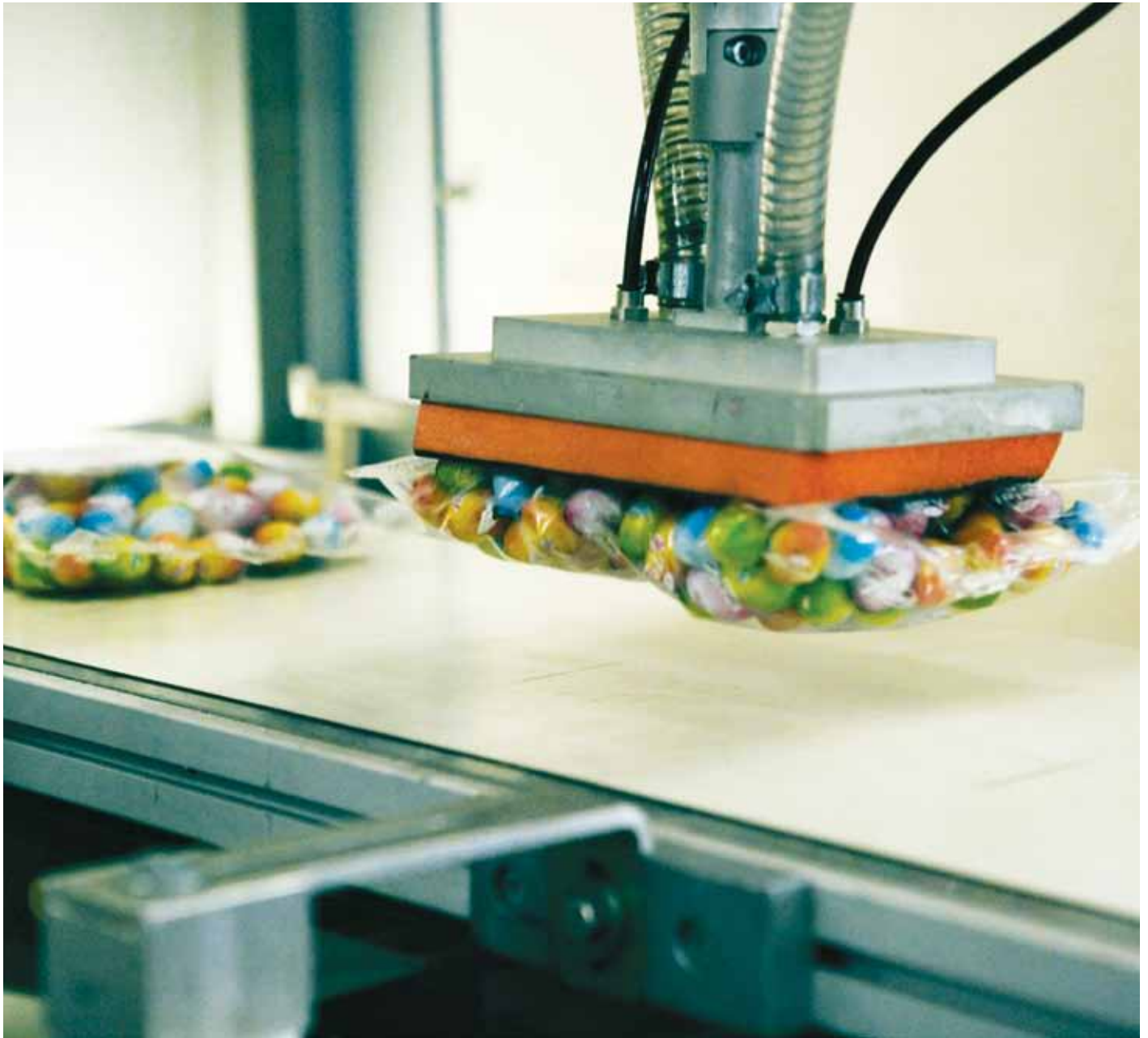
IRB 340 FlexPicker packing candy at Zaini's in Italy.
