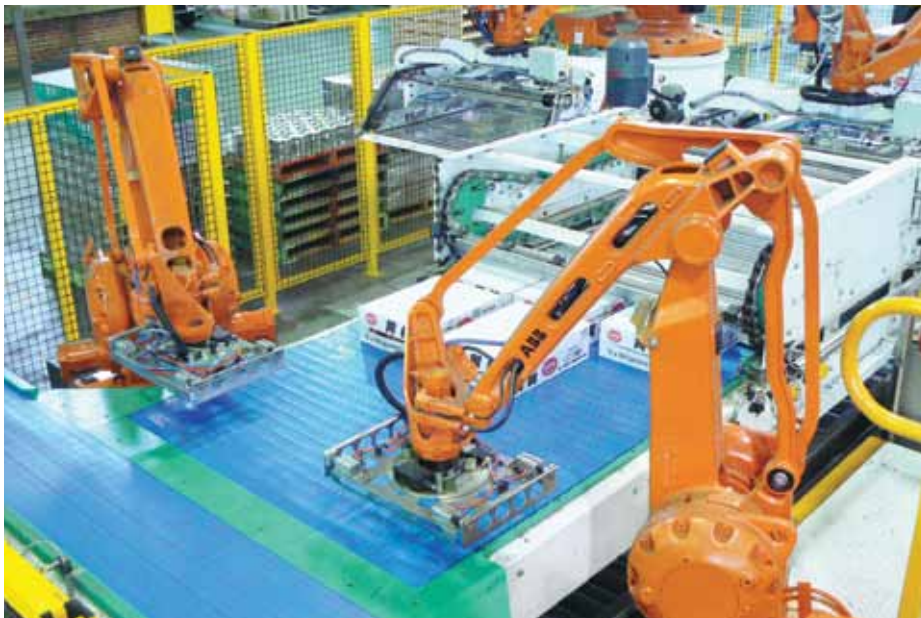
IRB 260 and IRB 660 robots packing and palletizing canned food at SPC Armona in Australia.
