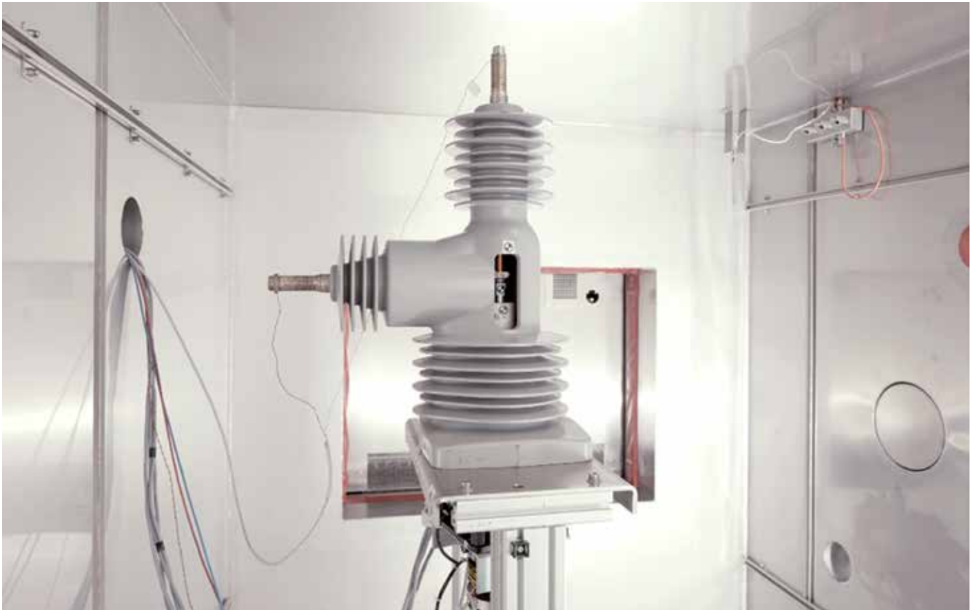
Figure 1: Climatic Testing and Validation – ABB 3-phase GridShield® recloser
