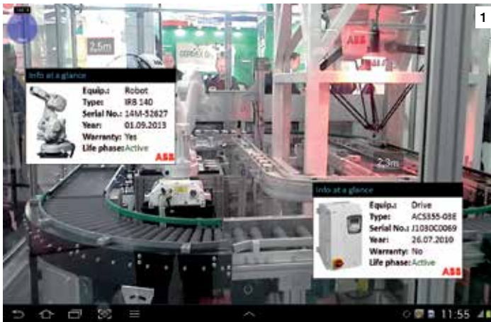
Figure 1: The prototype for demonstrating how devices can be localized within a plant or factory to provide more information | Figure 2: Main screen of the mobile app presenting wearable sensor data
