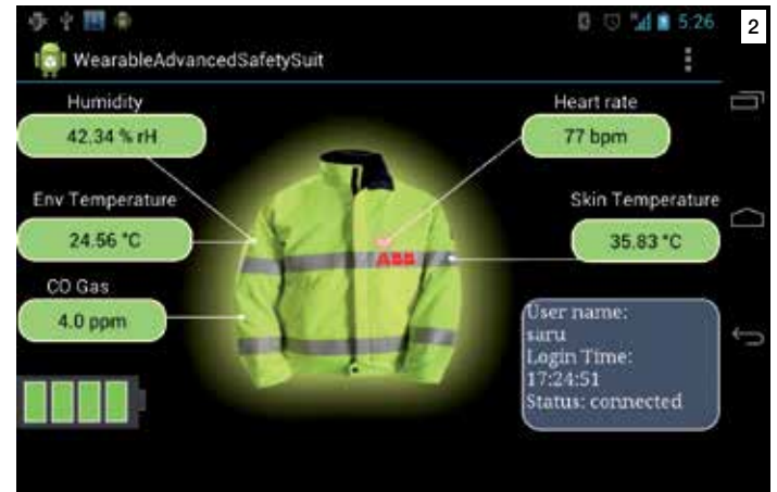
Figure 1: The prototype for demonstrating how devices can be localized within a plant or factory to provide more information | Figure 2: Main screen of the mobile app presenting wearable sensor data
