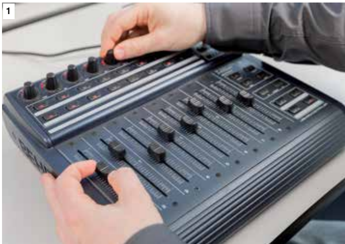
Figure 1: A MIDI controller that can be used to control multiple signal values live during simulation
