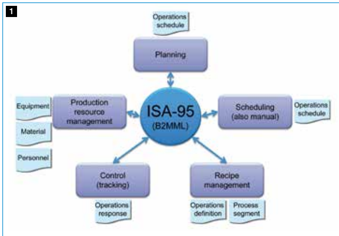
Figure 1: ISA-95 and B2MML elements providing full information required for scheduling. | Figure 2: Example of a workflow using B2MML data exchange. | Figure 3: Screenshot of the scheduling system. Above the typical Gantt-chart and below the trend curves for tracking electricity and material.
