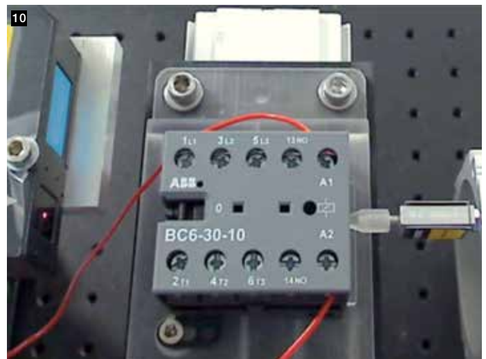
Figure 9: Low-voltage switching products are prime candidates for high-efficiency DEAs | Figure 10 Laboratory testing of low voltage switch [4]
