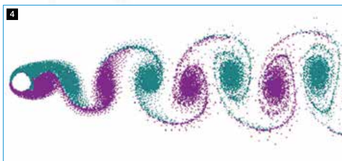
Figure 4: Alternating vortex shedding. The effect is also seen in a flag waving in the wind.
