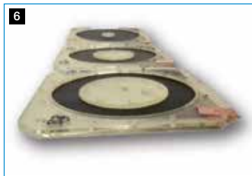
Figure 4: picture of a dielectric elastomer actuator (CT Systems) in stacked topology | Figure 5: schematics of a spring biased membrane actuator [4] Figure 6: picture of a dielectric elastomer actuator in membrane topology (here not spring biased) [4] | Figure 7: FEA Model of stacked dielectric elastomers in different geometries
