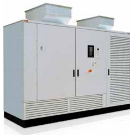
ABB's ACS1000i 3.3 kV medium voltage drive, uses a compact drive cubicle in which transformer, contactor and on-board auxiliary power supply are built-in.
