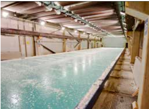
The ice tank is 75 meters long and 8 meters wide, with a water depth of up to 2.1 meters.
