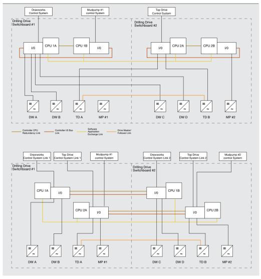
are doing parts of the calculation, requiring special attention to functional integration. A new unified power distribution module now allocates power in most configurations and interfaces. The module itself is the same, regardless of switchboard configurations. This means power limitation actions are more predictable and safer.
