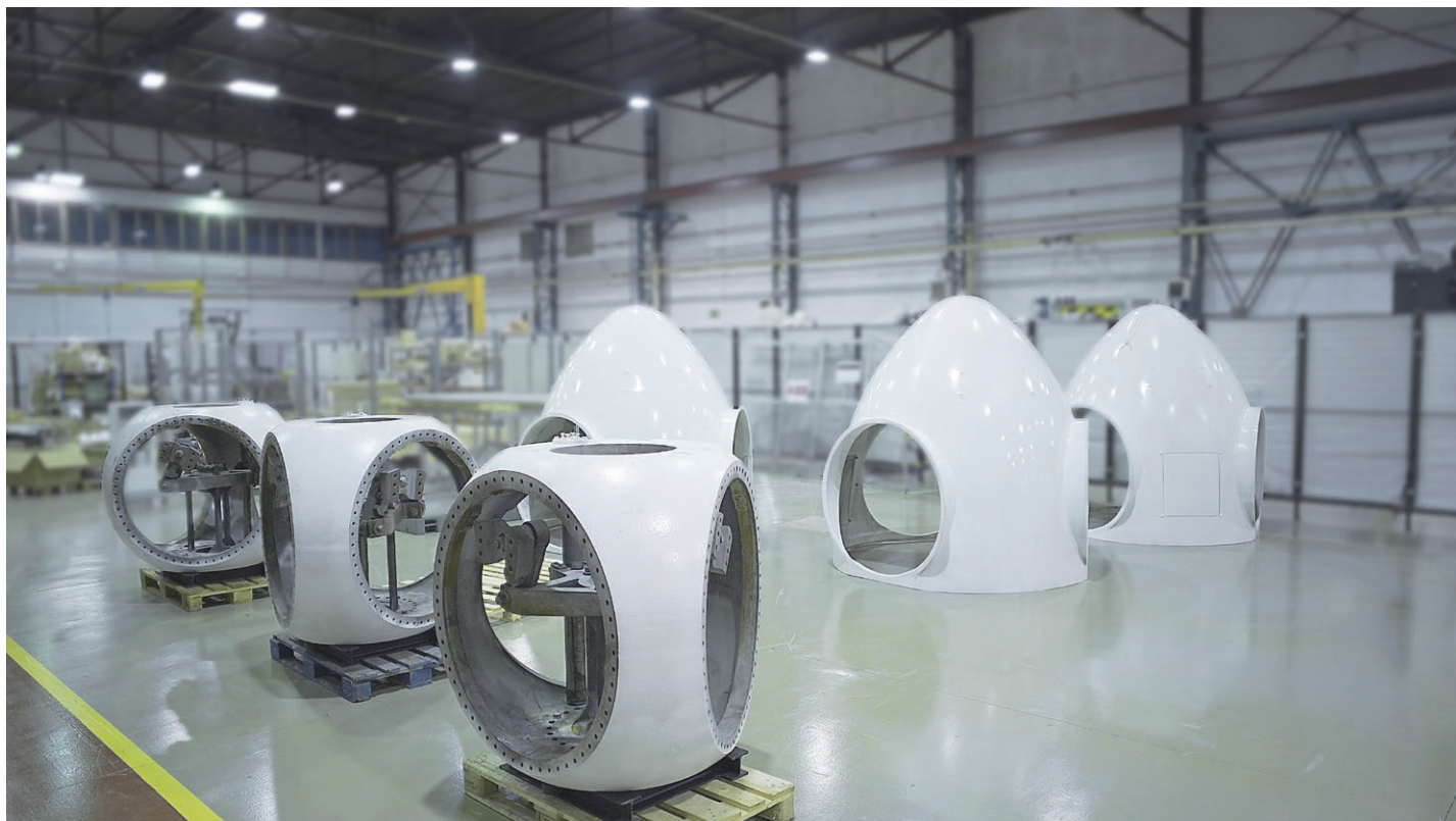
Wind turbine dismantled components to be remounted after the retrofit by ABB's Service Center of Excellence
