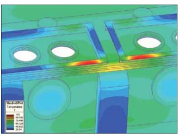
Thermovision of the LV turrets of an ABB 500 MVA single-phase GSU transformer (left), and the corresponding temperature distribution calculated by ABB (right).
