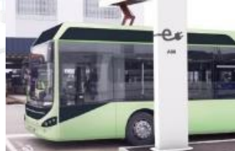
Flash-charging electric buses
