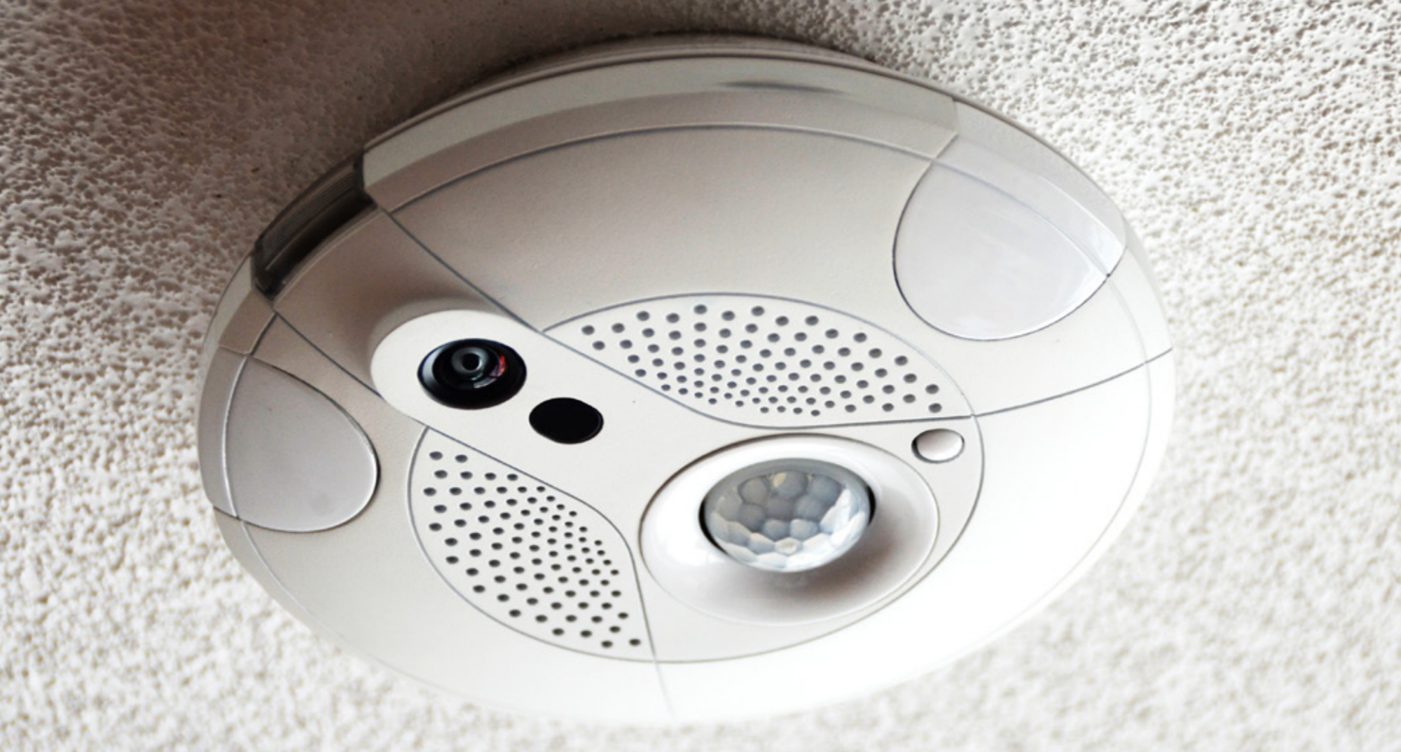
— 02 Pointgrab's vision sensor counts and tracks people without using CCTV but with similar accuracy.
