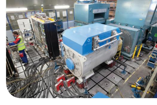
The test setup is self-powering, consuming its losses to drive the motors downstairs that run the testing rigs. Credit: ABB.
