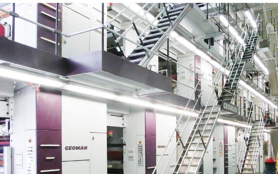
ABB has proven modular retrofit solutions for manroland Geoman presses. These eliminate problems with obsolete control systems, non-availability of spare parts and loss of production due to system failures – and the press doesn't even have to be taken out of production.
