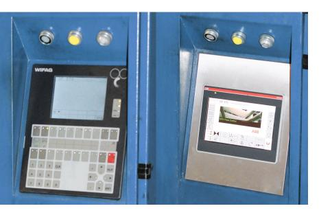
Owners of Wifag OFx70 presses (OF370, OF470 etc.) are confronted with the problem that the Lauer PCS950 displays used for the operator panels on their presses are obsolete and causing an increasing number of problems. ABB has now produced a 100% compatible operator panel based on the standard ABB CP635 display.
