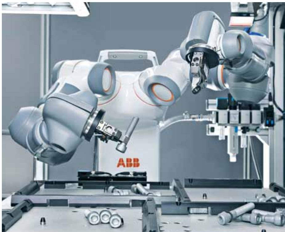
YUMI: ABB's Dual arm robot has sensor technology and can respond to the environment around it.
