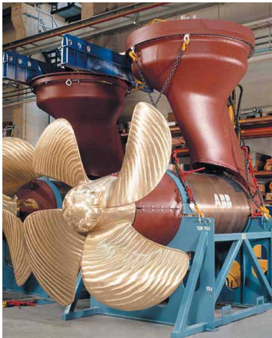
The Azipod thruster can reduce fuel consumption by 20%.
