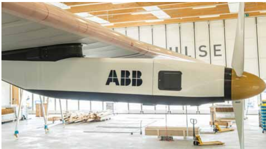
The Solar Impulse plane has 12,000 solar cells built in the wing providing four 10 HP electric motors with energy.
