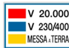
Sign for identification of the circuits with different colors for the different voltage levels and for the earthing conductors
