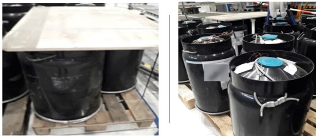
Figure 59. Reel 400/630 – 3 reels with a bell per pallet.
