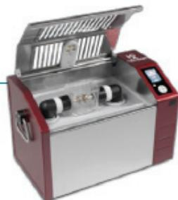
Breakdown Voltage Measurement
