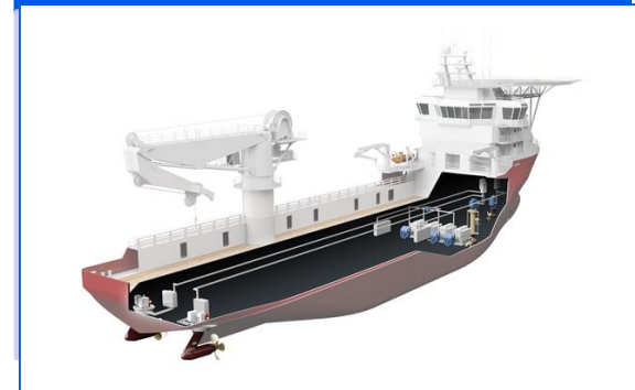
Power Generation and Distribution incl. DC Grid
