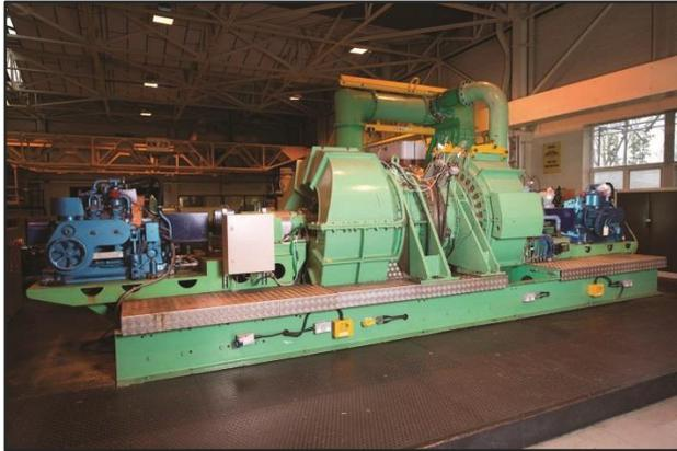
**Caption:** Alstom has cut the time needed to change its test rig set-up from six weeks to a few hours after the installation of an ABB VSD by Iconsys.
