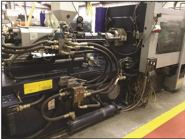
**Caption:** Atlantic Plastics is saving 20 percent of the energy costs of a large injection machine following the fitting of an ABB variable-speed drive.
