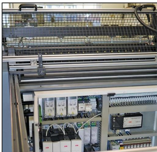
**Caption:** New plastic bag machine using ABB's Ethernet Powerlink compatible motion control.
