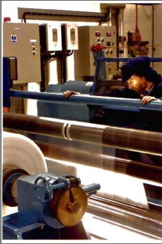
**Caption:** BPI Films is saving 66% of the energy on a slitter-rewinder machine for plastic film, following the installation of variable speed drives from ABB.
