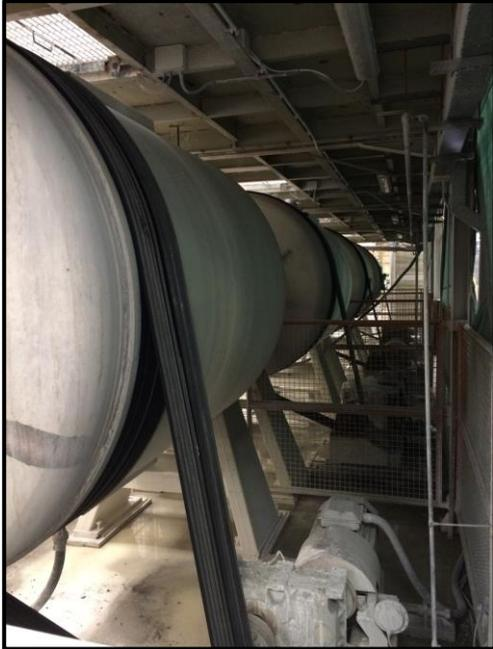
**Caption:** British Ceramic Tile has cut £4,800 per year from its energy bill following the replacement of a fluid coupling with a variable-speed drive on one of its glaze mills (pictured).
