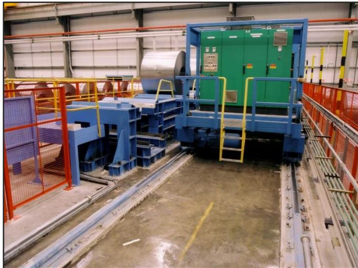
**Caption:** Two ABB drives, using fibre optic communications and Profibus DP, are helping Corus to accurately position two coil shuttle cars ahead of the hot dipping production lines.
