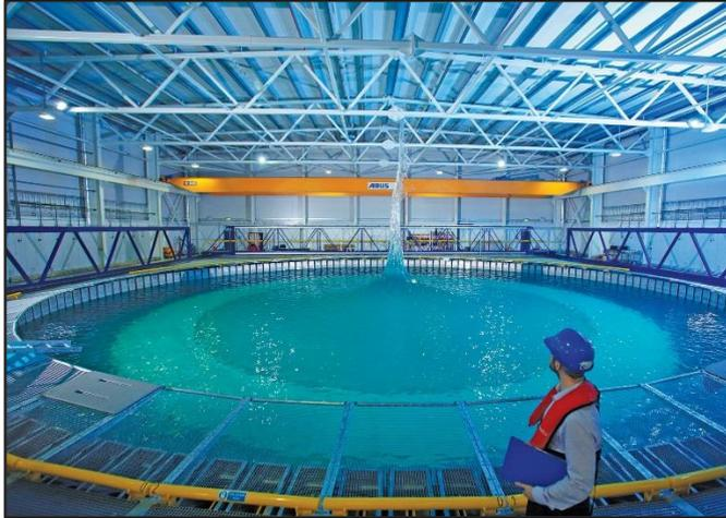
**Caption:** The world's first circular wave and tidal current test facility is using ABB electrical and control equipment to simulate energetic sea-states found in British, European and international waters.
