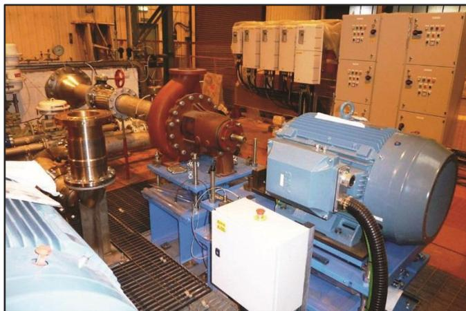
**Caption:** Flowserve is using ABB VSDs and motors for quick and easy testing of its new pump variants at different speeds.
