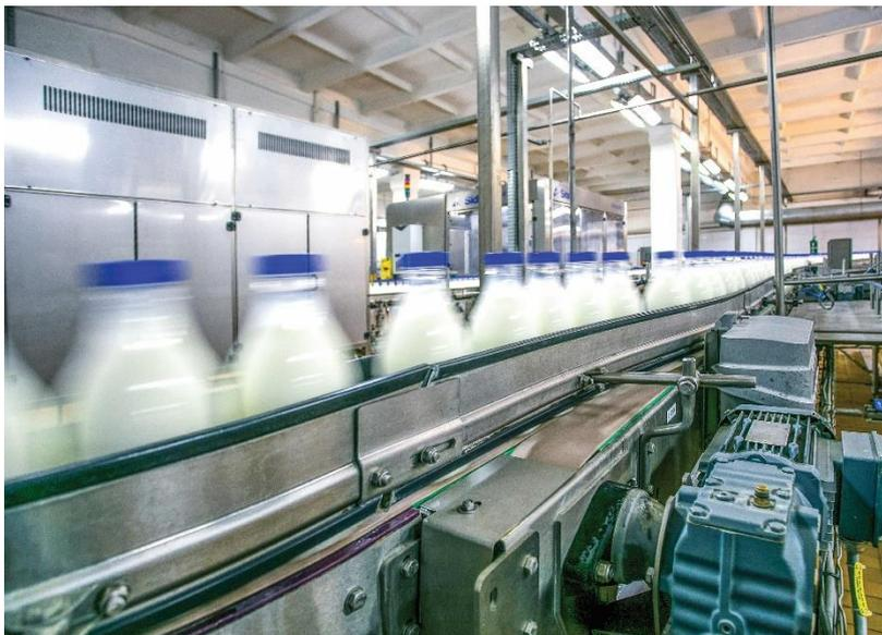
**Caption:** The compact size and low power rating range of ABB drives makes them an ideal fit for applications such as fans, pumps, mixers, conveyors, and compressors for food and beverage producers like Framptons (Image via Shutterstock)
