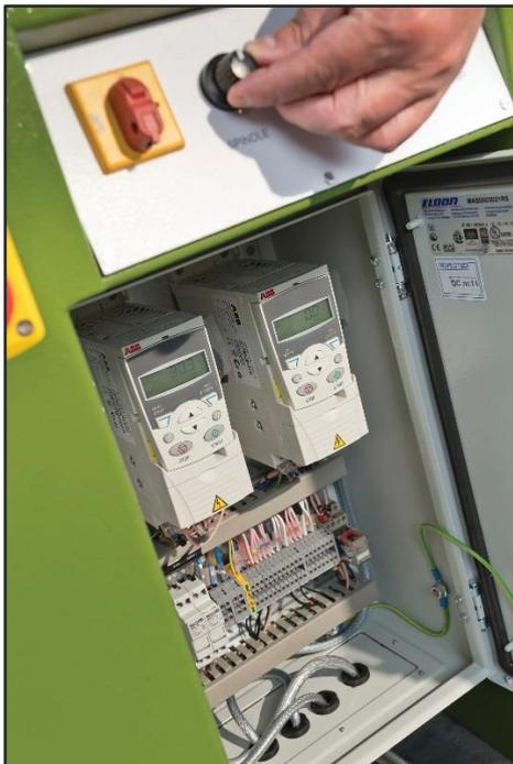
**Caption:** Panel containing two ABB machinery drives. One supplies the three-phase power and speed control for the milling machine, whilst the other provides three-phase power for the coolant pump.
