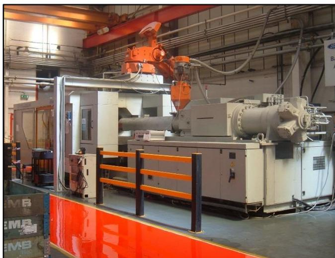
**Caption:** State-of-the-art controls based on a variable speed drive from ABB have cut the energy consumption by one third on an injection moulding machine at McKechnie Automotive and Engineered Plastics.
