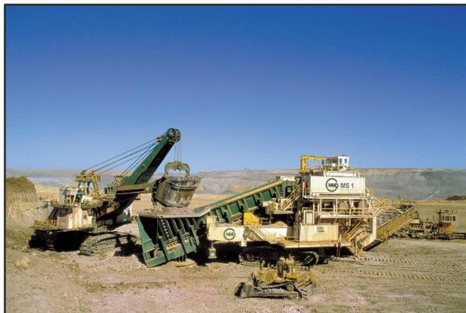
**Caption:** The world's largest mobile mineral crusher, used in open cast coal mining in Australia, is an all electrical piece of machinery, powered by ABB drives and motors.
