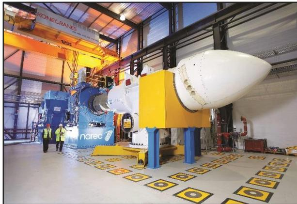
**Caption:** An ABB medium voltage drive and 12-pole motor are providing the motive power for a new test facility for proving marine energy generating systems.
