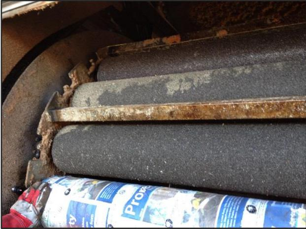
**Caption:** Maintenance intervals on a vegetable peeling machine are increased from four weeks to over six months by replacing standard bearings with ABB Dodge ISN bearings.
