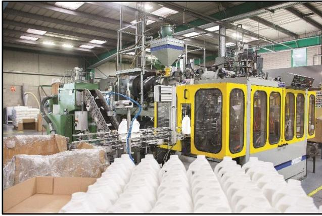
**Caption:** Before the installation of the ABB SynRM and drive package, only 63 percent of extrusions at the Northern Ireland plant became bottles. Now, 96 percent of extrusions are turned into bottles.
