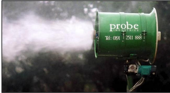
**Caption:** The revolutionary Rotary Atomiser, made by Probe Industries, which removes dust and odours from the atmosphere uses ABB variable speed drives supplied by Drives Alliance partner Slater Drives Systems.
