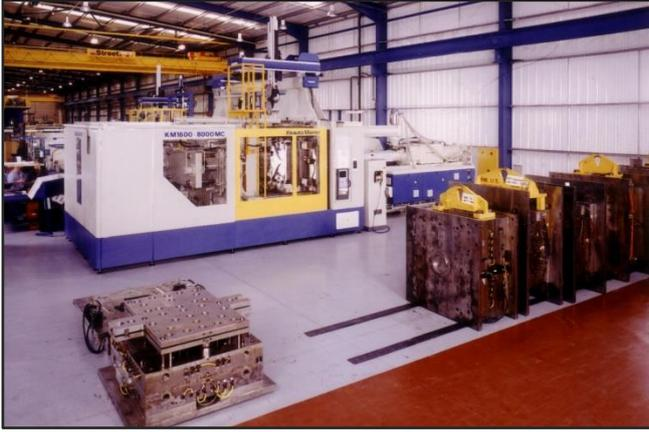
**Caption:** Controlling the hydraulic system with variable speed drives from ABB is helping to save £10,000 per year on the energy consumption of R-TEK's injection moulding machines.
