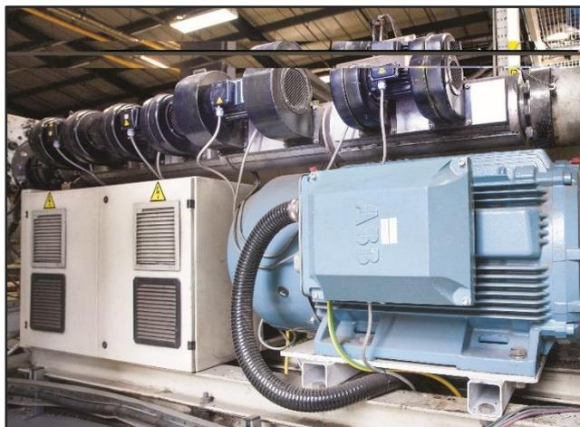
**Caption:** An ABB synchronous reluctance motor and drive package has cut energy consumption on a twin extruder application by up to 15 percent, reducing maintenance costs and noise.
