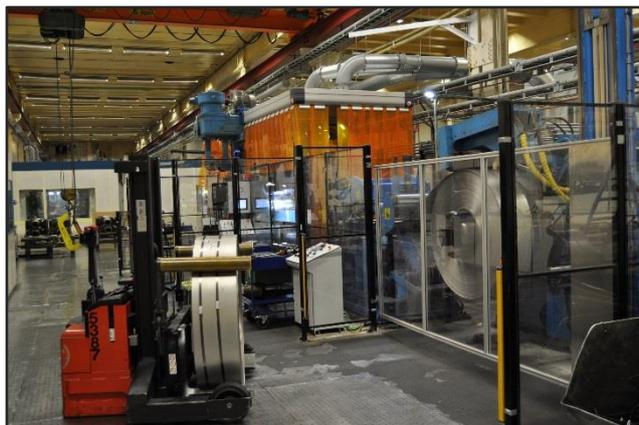
**Caption:** ABB's safety PLC controls gate switch and light curtain guarding emergency stop buttons and other safety features on Sandvik's 20 M long stainless steel rolling mill.
