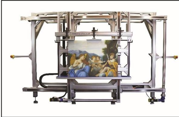
**Caption:** SmartDrive's SatScan uses ABB's motion controllers for the accurate positioning and movement of digital scanners.
