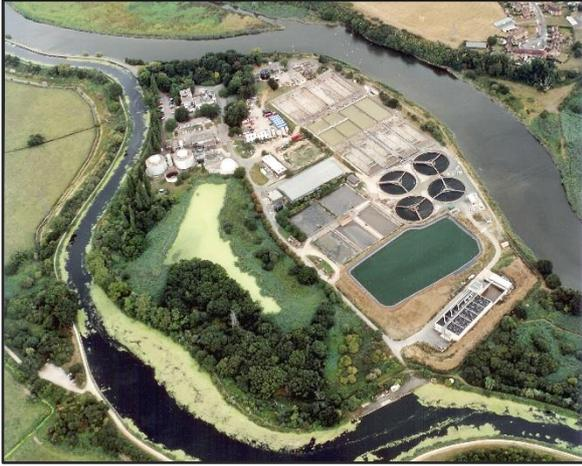
**Caption:** Low harmonic ABB drives have allowed the Countess Wear waste water treatment works, south of Exeter, to increase its pumping capacity without causing disturbances on the electrical supply network.
