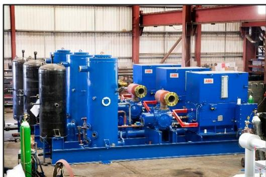
**Caption:** Six ABB medium voltage motors are providing the compression stage for the world's largest district-wide natural heat pump system.
