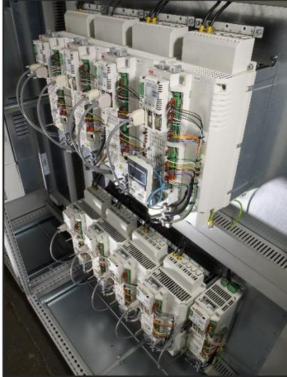
**Caption:** ABB and Tatham have developed control software based on ABB high performance machinery drives' programmable function blocks which provide precise positioning.
