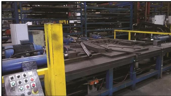
**Caption:** voestalpine Metsec is saving 28 percent on its energy bill after retrofitting an ABB variable speed drive on a metal bending machine.
