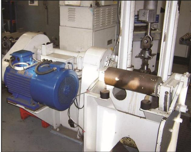
**Caption:** Quieter and higher reliability has been achieved for Wabtec Rail by fitting ABB variable speed drives to a damper tester used in the upgrade and refurbishment of railway equipment.
