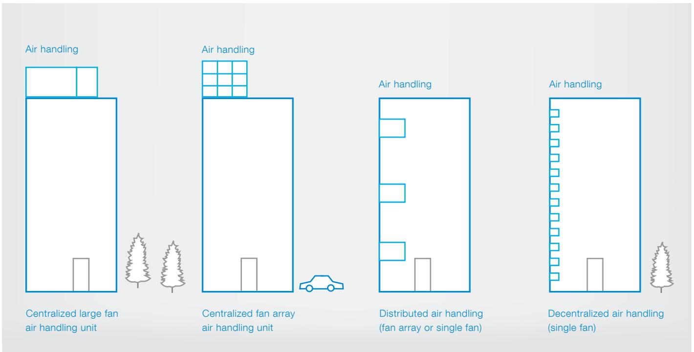
Four different ways to handle air handling in a building.
