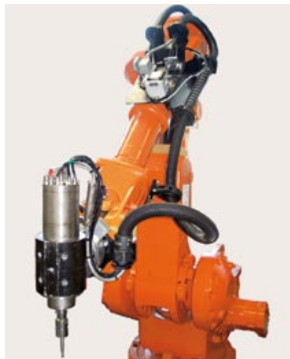
Obr.3 Robot s Force Control Function package (softvér na riadenie sily)
