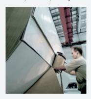
Cut the sample (different cutter models are available as options depending on grades and environment).
